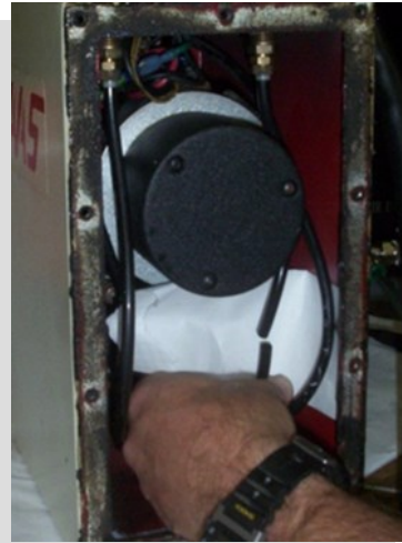
3. Cut this hose in half as close to the opening of the box as possible and attach quick disconnect "T" (provided)
