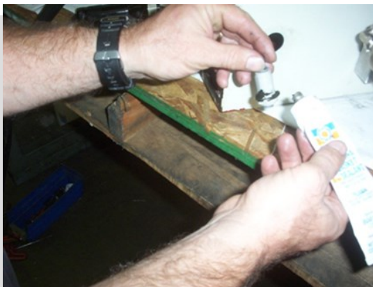
5. Insert bulkhead fitting (provided). Spread permatex around inside of flange on both sides (permatex provided)
