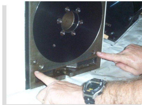
6. Mount pump to back of indexer using (2) cap screws (provided)
