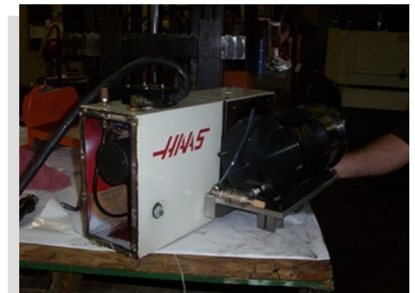
7. Connect 1/4" hose from air inlet port side (as shown on back of cylinder)
